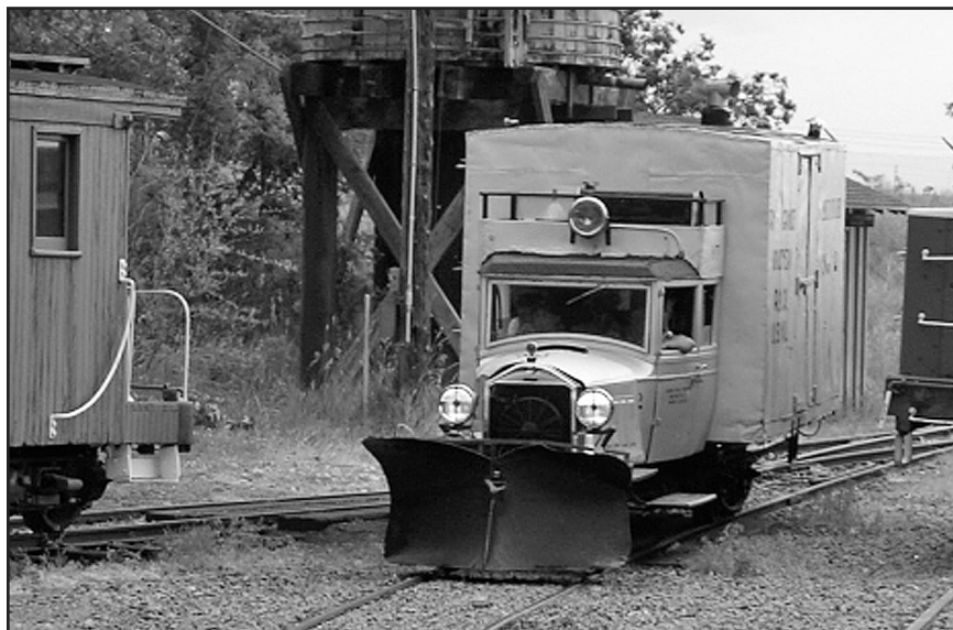
RGS motor car number 2 paced the CRRM Fathers day weekend train at a safe distance all day, June 17th. Goose 2 was taken out of service a few years ago because the flanges on the drive wheels were severely worn. New wheels were cast and along with a lot of care to the cab and some new brakes RGS 2 was back in action. – Photo © 2007 Denny HaefeLe.
